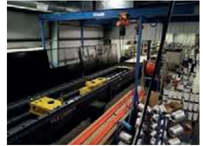
Yale Cordage will use the test bed for destructive and non-destructive testing of rigging gear.
