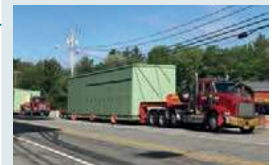
The 3-axle trailers on air suspension are rated for 100,000 pounds technical capacity.
